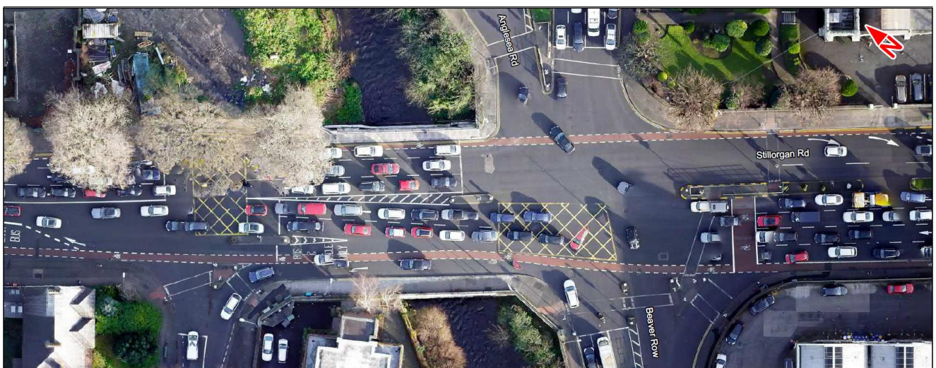
Image 5.15: R138 Donnybrook Road / R815 Anglesea Road Junction Four-arm Signalised Junction Arrangement
