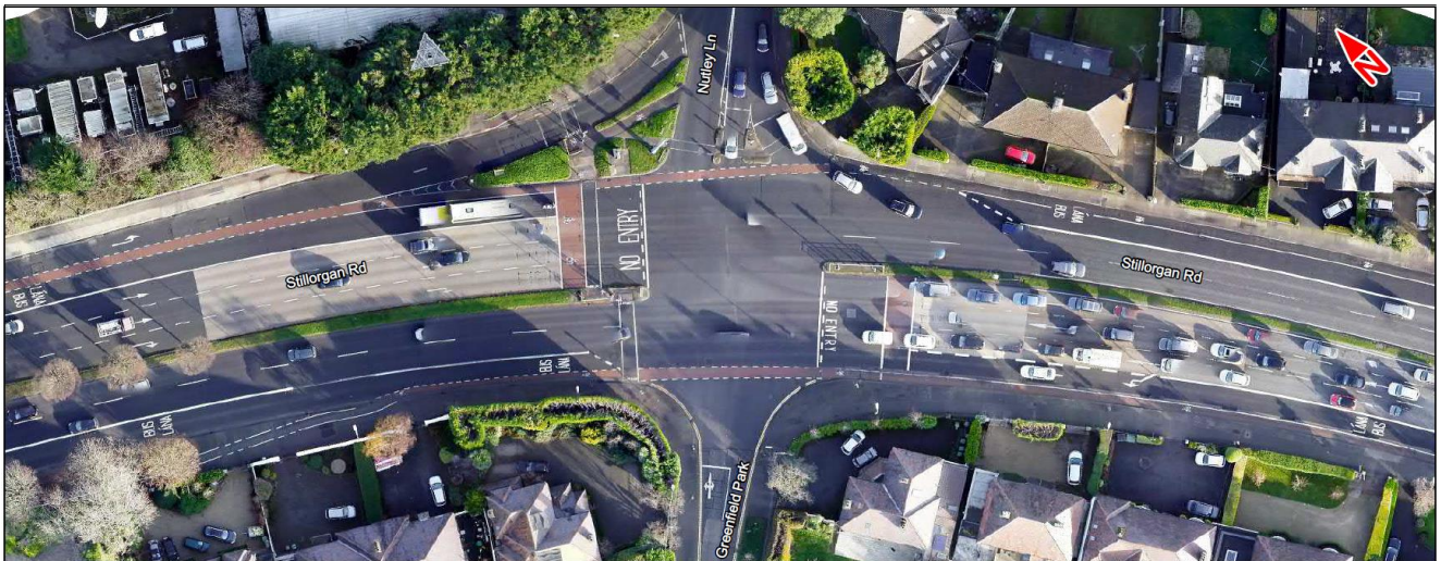
Image 5.17: R138 Stillorgan Road / Nutley Lane Four-arm Signalised Junction Arrangement (Source: OSI)
